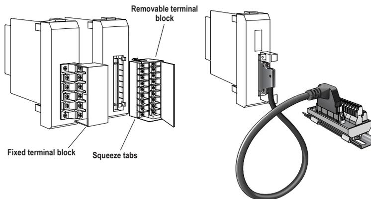
**ZIPLinks eliminate the tedious process of wiring PLC I/O terminal blocks.**
