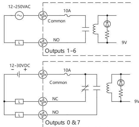
\* Caution: the ZIPLink wiring system is rated at 2 Amps per I/O point and 4 Amps per common, therefore the D3-08TRS-1 relay outputs are derated to 2 Amps per point and 4 Amps per common when used with the ZIPLink wiring system.
