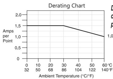
**Derating Note:** All outputs can be run at the current per point shown.
