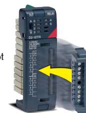
16 pt module with removable terminal block
