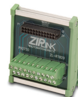
ZL-RTB20 20-pin feed-through connector module
