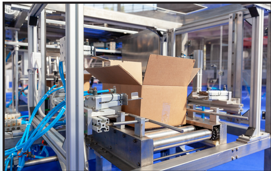
Cardboard case erector using T-slotted aluminum rail for support and mounting working components
