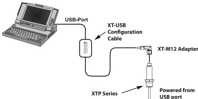
Note: XT-SOFT version 1.27.13.0 or later required for use with the XTP series transmitters
