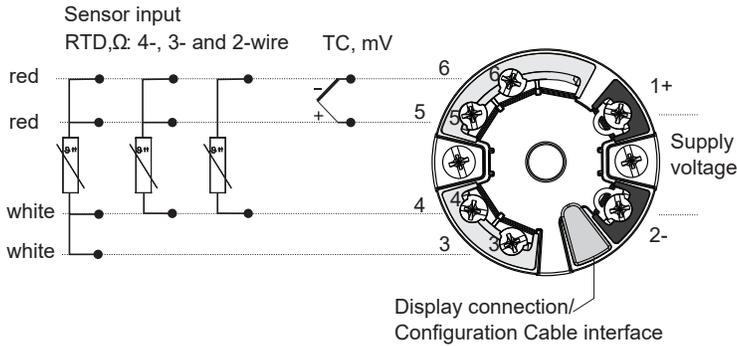
Note: In the event of a thermocouple (TC) measurement, a 2-wire Pt100 RTD can be connected to measure the reference junction temperature. This is connected to terminals 4 and 6.
