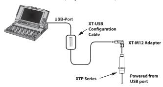
Note: XT-SOFT version 1.27.13.0 or later required for use with the XTP series transmitters
