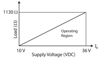
$$R_{Lmax} = (V_{powersupply} - 10V) / 0.023A \text{ (current output) e.g. } (24V - 10V) / 0.023A = 608.7 \Omega$$
