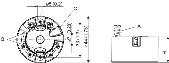
Head transmitter version with screw terminals.
