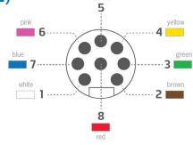
**NOTE:** The colors used in this connection chart are for 292 series 8-pin cables.
