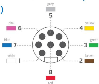
**NOTE: The colors used in this connection chart are for 292 series 8-pin cables.**
