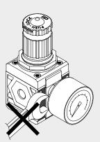
Do not use a spanner for fixing taper threaded elements to the front ports. Mount by hand and apply a liquid sealant (not teflon<sup>®</sup>).
