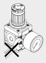
Do not use a spanner for fixing taper threaded elements to the front ports. Mount by hand and apply a liquid sealant (not teflon®).
