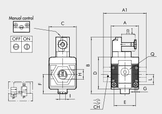
**N.B.**: Before assembling other Syntesi elements after the APR, remember to mount the coil on the APR itself.
