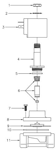
Special Note – Older units may require a GCV Spanner Nut Tool (106198E) or spanner wrench to remove the plunger tube base nut. Consult your distributor or call GCV customer service for assistance.
