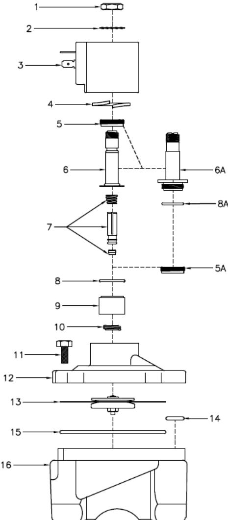
**Special Note – Valves constructed with Nylon bodies do not have Item 9 installed.**
