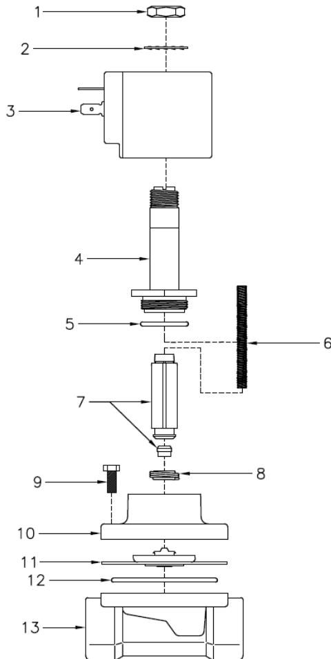
**Special Note – Older units may require a GCV Spanner Nut Tool (106198E) or spanner wrench to remove the plunger tube base nut. Consult your distributor or call GCV customer service for assistance.**
