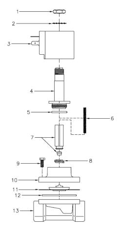
Special Note – Older units may require a GCV Spanner Nut Tool (106198E) or spanner wrench to remove the plunger tube base nut. Consult your distributor or call GCV customer service for assistance.
