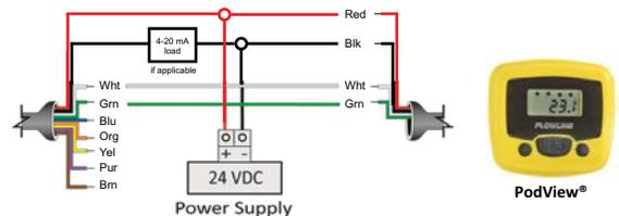
Note: Maximum distance between EchoPod sensor and PodView display is 15 ft. (4.5m)
