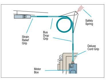
CAUTION: Never use grip to approximate breaking strength. Refer to technical data page for safety and working load factors. Banding is necessary to guard against accidental release of grip and provide maximum reliability.
