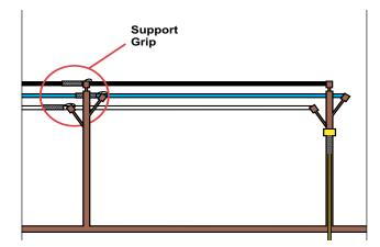
CAUTION: Never use grip to approximate breaking strength. Refer to technical data page for safety and working load factors. Banding is necessary to guard against accidental release of grip and provide maximum reliability.
