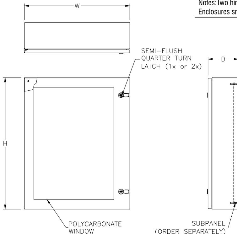
Notes: Two hinges are provided when H=36 in [914 mm] with each enclosure. Enclosures smaller than 24 in [610 mm] have one latch.
