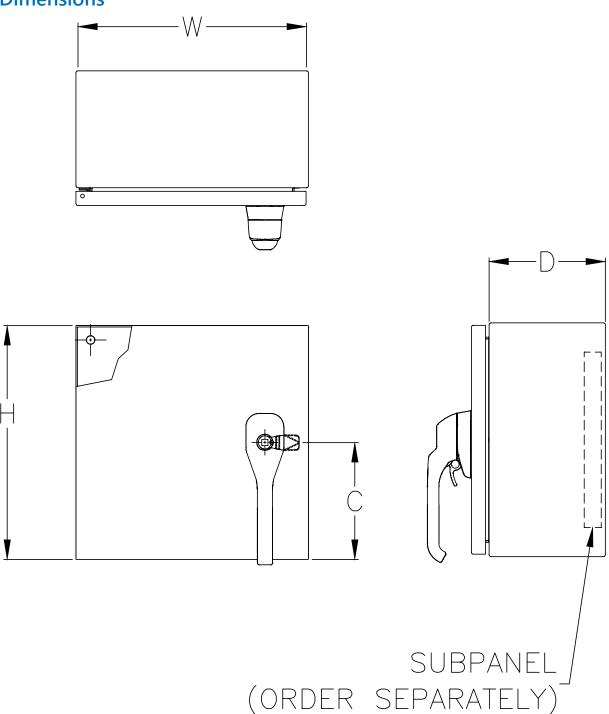
Notes:Two hinges are provided when H=36 in [914 mm]. Three hinges are provided when H=36 in [914 mm] or greater. Four hinges are provided when H=48 in [1219 mm] or greater.
