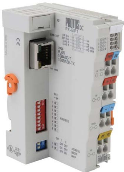
The PX-EIP1 EtherNet/IP Bus Coupler server allows connection of up to 64 terminals per assembly, 255 terminals total with I/O bus expansion. The PX-EIP1 module has one RJ45 Ethernet 10/100 Base T port for connection to an Ethernet client. Use with the Protos X I/O System.
