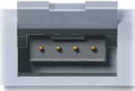
The Service Port connector is located under the flip-cover shown. This port is used for communication with the software configuration tool. The software configuration tool autoconfigures the Modbus addresses of the I/O terminals and the interface allows the user to:
