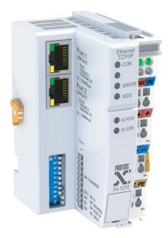
The PX-TCP2 Modbus TCP Server Bus Coupler allows connection of up to 64 terminals in a Modbus TCP network. The PX-TCP2 communicates using high-level Modbus commands and supports 512 bytes of input data and 512 bytes of output data.
