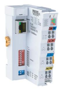
The PX-TCP1 Modbus TCP Server Bus Coupler allows connection of up to 64 terminals per assembly, 255 terminals total, in a Modbus TCP network. The PX-TCP1 communicates using high-level Modbus commands and supports 512 bytes of input data and 512 bytes of output data.
