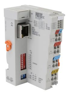
The PX-EIP1 EtherNet/IP Bus Coupler server allows connection of up to 64 terminals per assembly, 255 terminals total with I/O bus expansion. The PX-EIP1 module has one RJ45 Ethernet 10/100 Base T port for connection to an Ethernet client. Use with the Protos X I/O System.
