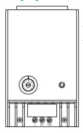
Notes: Only connect the L and N1 terminals – N2 is not used and Grounding is not required. When wiring 230 volt units for North American installations "L" (line) and "N" (neutral) will be used as "L1" (line1) "L2" (line2) respectively with no neutral connection.
