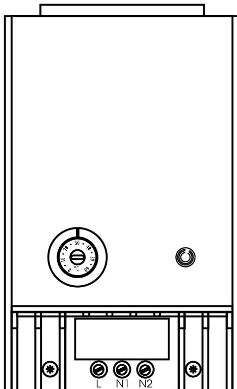
Notes: Only connect the L and N1 terminals – N2 is not used and Grounding is not required.
