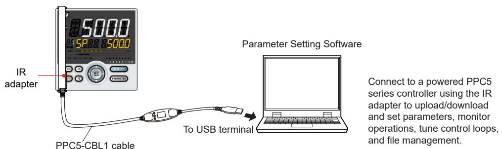
The IR adapter does not power the controller.
