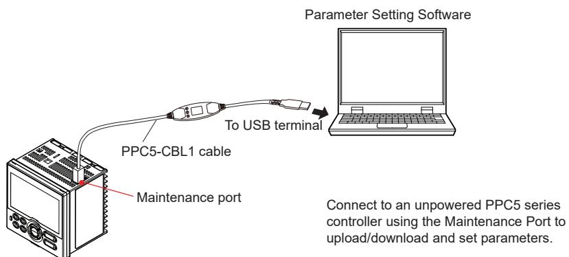
When using the maintenance port, power is provided from the USB port. Do not supply power to the controller through the terminals until disconnected from the maintenance port.
