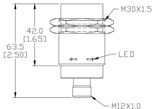
See our website: [www.AutomationDirect.com](http://www.AutomationDirect.com) for complete Engineering drawings.
