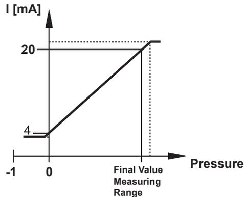
In the measuring range the output signal is between 4 and 20mA. If the system pressure is above or below the measuring range, the analog output performs as follows:
