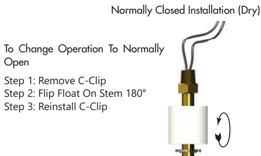
Figure 1: Vertical (Top) Mount Switch Operation
