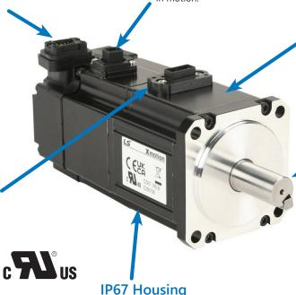
All LS Electric FBL motors have keyed shafts for use with servo-grade clamp or compression couplings (recommended) or servo-grade keyed couplings. Some sanding/filing of the key may be required before pressing into the keyway. Do not modify the shaft/keyway.
