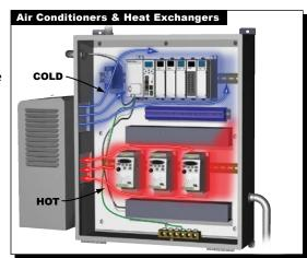
If the ambient air temperature is too high, and a source of chilled water is available, then an air-to-water heat exchanger may be the ideal solution. Air-to-water heat exchangers use fans to blow across tubes with chilled water running through them. This creates a very effective closed loop cooling effect, but requires an external source of chilled water.
