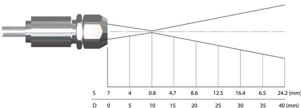
*Optical chart CSMicro LT (15:1) with CF lens (0.8 mm @ 10mm)/ D:S Far field = 1.4:1*
