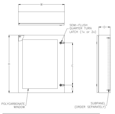
Notes:Two hinges provided with each enclosure. Enclosures smaller than 24 in [610 mm] have one latch.
