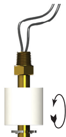
Figure 1: Vertical (Top) Mount Switch Operation
