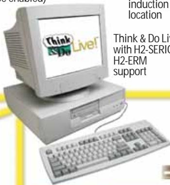
PC controls sortation machine and has HMI and motion control. Tracks packages from induction to diverting location
