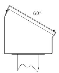
CONSOLET CAN BE POSITIONED AT 30° OR 60° ANGLE
