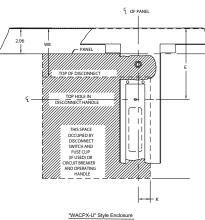
When ordering 24.13 (613mm) deep enclosures, long connecting rods must be ordered. Long connecting rods are available from disconnect manufacturers.
