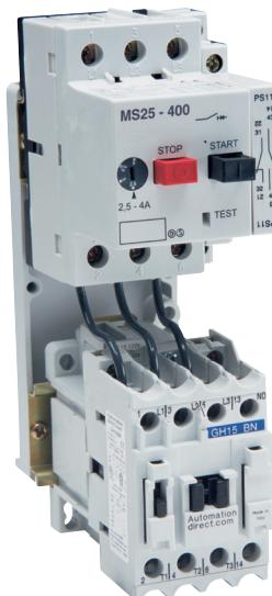
Motor starter/protector combination consisting of a contactor, MSP with optional MS25-PS11 auxiliary contact and a UMP45 adapter plate. Components are sold separately.
