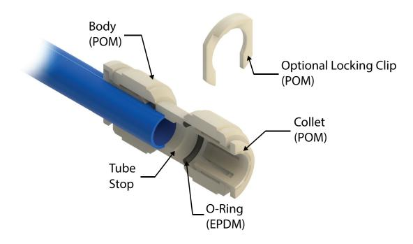
Push-to-Connect Fitting Cut-away Diagram
