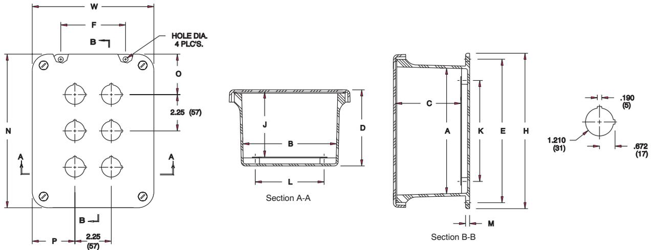
Dimensions for 30mm Multi-Hole Pushbutton Series with Lift-off Cover
