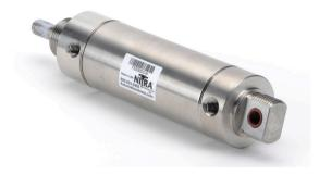
NITRA pneumatic stainless steel round body, interchangeable, non-repairable cylinder, 2 inch bore, 1/4 inch female NPT ports, double acting, double end mount, magnetic piston.
