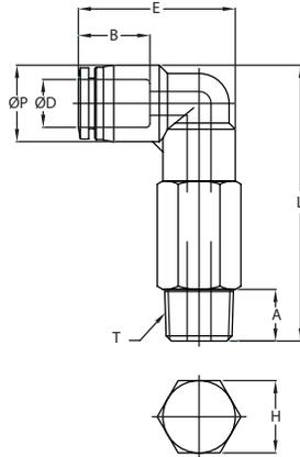
**NITRA** pneumatic push-to-connect long male elbow fitting with rotating thermoplastic (PBT) body, nickel-plated brass threads, stainless steel tube gripping claws and pre-applied Teflon thread sealant (O-ring on #10-32 and M5 threads). For use with polyurethane or nylon tubing. Five fittings per package.
