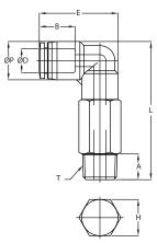
**NITRA** pneumatic push-to-connect long male elbow fitting with rotating thermoplastic (PBT) body, nickel-plated brass threads, stainless steel tube gripping claws and pre-applied Teflon thread sealant (O-ring on #10-32 and M5 threads). For use with polyurethane or nylon tubing. Five fittings per package.
