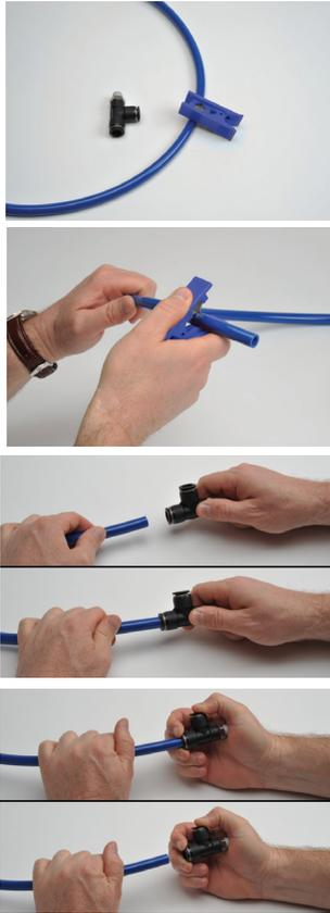
Prepare the **NITRA** tubing for cutting and make sure to have the proper tubing cutters like the **NITRA** TC-12 or TC-20.
