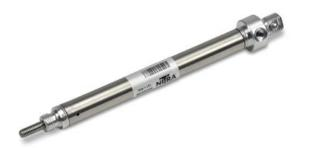
NITRA pneumatic stainless steel round body, interchangeable, non-repairable cylinder, 7/16 inch bore, #10-32 port, single acting, spring return, rear pivot mount (pivot pin included).
