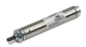
NITRA pneumatic stainless steel round body, interchangeable, non-repairable cylinder, 3/4 inch bore, 1/8 NPT port, single acting, spring return, front nose mount.
