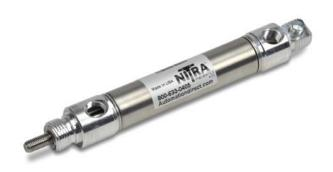
NITRA pneumatic stainless steel round body, interchangeable, non-repairable cylinder, 3/4 inch bore, 1/8 NPT ports, double acting, rear pivot mount (pivot pin included), magnetic piston.
