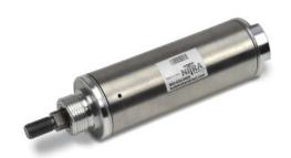
NITRA pneumatic stainless steel round body, interchangeable, non-repairable cylinder, 2 inch bore, 1/4 NPT port, single acting, spring return, front nose mount.
