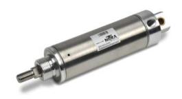
NITRA pneumatic stainless steel round body, interchangeable, non-repairable cylinder, 2 inch bore, 1/4 NPT port, single acting, spring return, double end mount.
