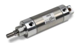
NITRA pneumatic stainless steel round body, interchangeable, non-repairable cylinder, 2 inch bore, 1/4 NPT ports, double acting, double end mount
