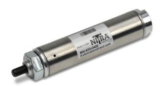
NITRA pneumatic stainless steel round body, interchangeable, non-repairable cylinder, 1-1/16 inch bore, 1/8 NPT port, single acting, spring return, front nose mount.
