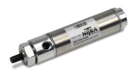
NITRA pneumatic stainless steel round body, interchangeable, 1-1/16 inch bore, 1/8 NPT ports, double acting, front nose mount.
