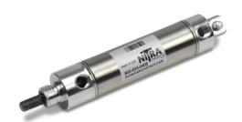
NITRA pneumatic stainless steel round body, interchangeable, 1-1/16 inch bore, 1/8 NPT ports, double acting, rear pivot mount (pivot pin included).
