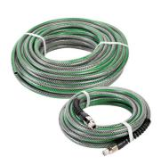
NITRA™ Hybrid PVC hose is a blend of PVC and rubber with a polyester braided reinforcement. The PVC gives light weight, color stability and hardness for higher working pressures while the rubber gives improved flexibility and operating temperature range. Our Hybrid PVC polyester reinforced hose is sold with or without male NPT nickel-plated brass rigid fittings (additional fittings may be purchased separately).
