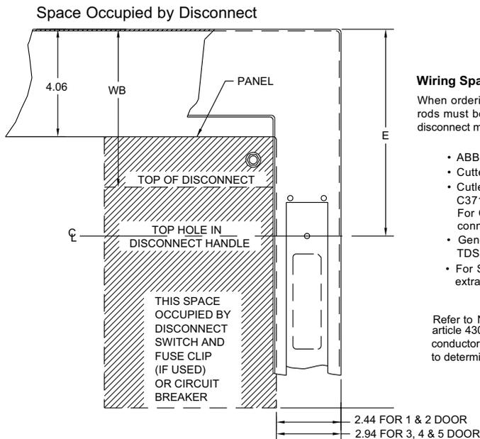
**Wiring Space "WB" is available when disconnect is installed in the enclosure.**
