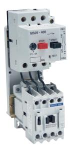
Motor starter/protector combination consisting of a contactor, MSP with optional MS25-PS11 auxiliary contact and a UMP45 adapter plate.
