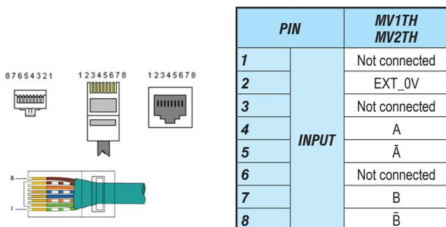
**NOTE: All inputs must be utilized. For example, an encoder without the  $\bar{A}$  signal will not work. Be sure to select a compatible encoder type.**
