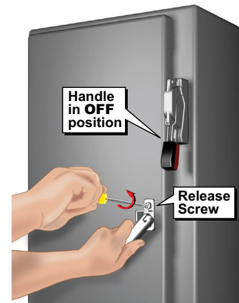
Safety Handle shown on enclosure
