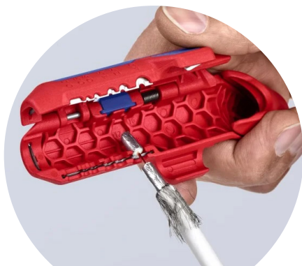
Dismantling and stripping of coaxial cables
