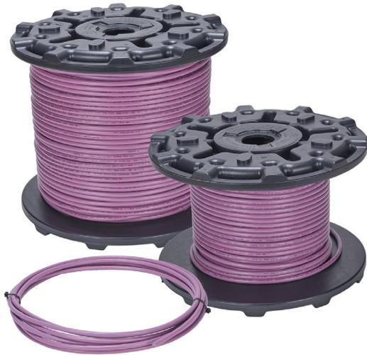
AutomationDirect is pleased to offer the igus CFBUS series PVC cable for continuous flexing applications. This cable is available in a 24AWG twisted pair. Individual conductors are bare copper and stranded for flexing applications. Conductor insulation is a mechanically high-quality red and green TPE mixture. The cable's outer jacket is a low-adhesion pressure extruded Purple PVC mixture that provides resistance to sunlight, oil penetration, and is flame retardant.
