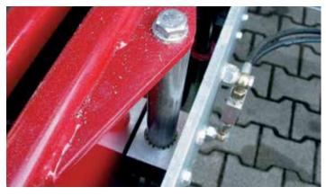
This saw mill uses a DryLin<sup>®</sup> linear bearing with iglide<sup>®</sup> J plastic liner for the angle stops.
