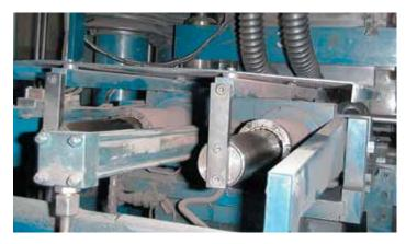
Despite the high stresses from abrasive particles and powder particles, this compactor unit can extend maintenance-free uptime by up to two years after switching to DryLin<sup>®</sup> R linear bearings.
