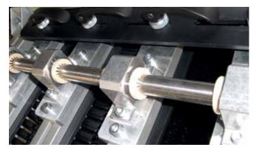
To enable fast, and precise adjustment of a production line without the need for downtime, DryLin<sup>®</sup> precision linear guides were utilized.
