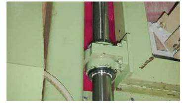
This heavy duty application has run reliably for more than three years thanks to DryLin<sup>®</sup> RJUM-01 linear bearings
