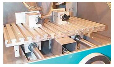
DryLin<sup>®</sup> R linear plain bearings on supported aluminum shafts are used in the guide for this cutting table. The DryLin<sup>®</sup> components stand up to the high levels of dust and dirt, and offer accurate, smooth operation.
