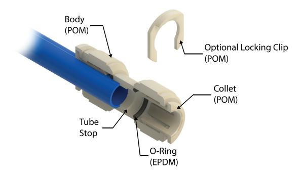
Push-to-Connect Fitting Cut-away Diagram
